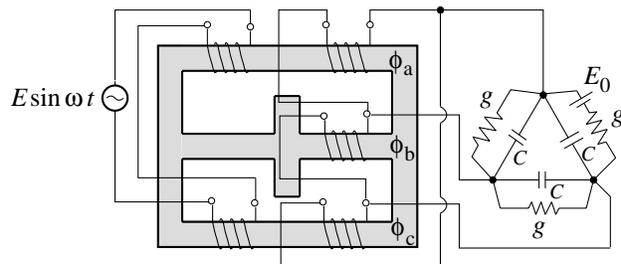
Figure 1: A phase converter circuit.
