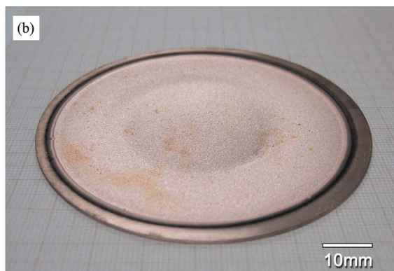
FIG. 3. (Color online) Erosion on the metal conductor (Cu) target. (a) and (b) show a profile and a photo of the erosion on the surface. The condition of the sputtering was high frequency electricity (200 W), and the accumulated electric discharge time was 150 h. A typical single circular erosion pattern was confirmed on the target.
