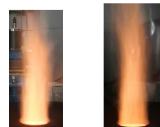
Figure 3 Single NH 3 firing for carbon-free technology. Premixed: 7m/s Premixed: 9m/s
